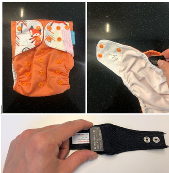
Fig. 1 Placement of the Axivity AX3 accelerometers in the diaper pants (upper panel) and wristband (lower panel)
